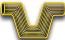
FORGED GRAIN STRUCTURE
