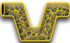
CAST GRAIN STRUCTURE
