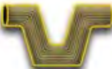
FORGED GRAIN STRUCTURE
